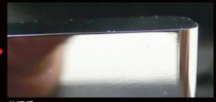
通过熔接修补后的研磨得以修复
